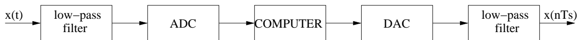
Figure 3: Low-pass filters in a digital audio system ensure that signals are bandlimited.
